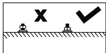
Using a second person to assist you, place Bench Top (A) upside down onto a padded, non-marring surface. Position and secure Legs (B) to Bench Top (A) with eight (two per leg) Nuts (H-1), Spring Washers (H-2) and Flat Washers (H-3) using the provided Open Wrench (T-1), stacking the hardware in the order as shown. DO NOT OVERTIGHTEN.
