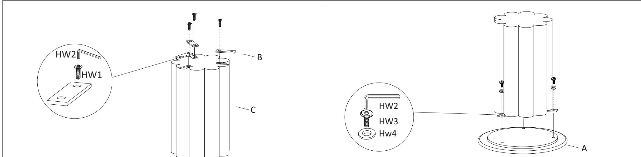
**STEP 1:** Put the base (C) on a flat surface. Align the screw holes on the assembly plate (B) to the base (C). Use the Allen key (HW2) to screw in the bolts (HW1) as shown in the picture.
