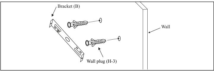
Place Bracket (B) on the wall at your desired location. Ensure the power cord will reach an outlet. It is suggested to use a Level (T-2; not included) to ensure the product is level. Mark the locations of the through holes onto the wall. Pre-drill holes on marked location using a Power Drill (T-3; not included) and a drill bit roughly the same diameter of the Wall Plugs (H-3). Insert the Wall Plugs (H-3) into the pre-drilled holes until they are roughty flush with the surface of the wall.
