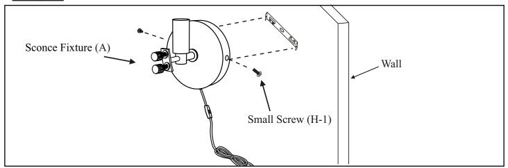
Place the Sconce Fixture (A) over Bracket (B) so that the side holes align with one another as shown. Insert Small Screws (H-2) into the side holes and tighten with a Screwdriver (T-1, not included). Check your work and that all connections have been fully tightened.
