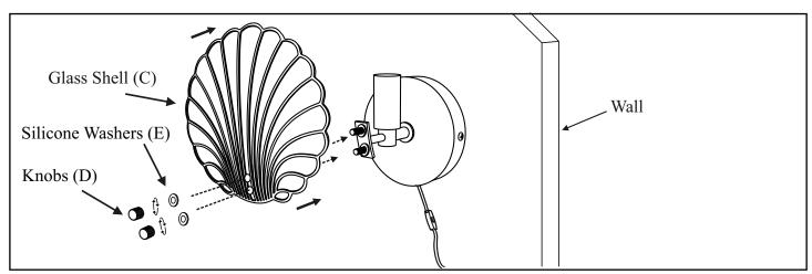
Remove the Knobs (D) from the Sconce Fixture (A) by unscrewing them counter clockwise. Place the Glass Shell (C) onto Sconce Fxture (A) and insert the bolts through the receiving holes and attach Silicone Washers (E) onto Glass Shell (C) Secure by re-attaching the Knobs (D). DO NOT OVERTIGHTEN.
