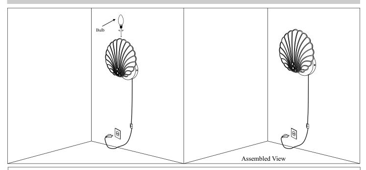
Insert Bulbs (not included) into the socket and rotate it in clockwise to secure. Restore power to the circuit at this time and check for proper lighting operation. Assembly is now complete and the product is ready for use.
