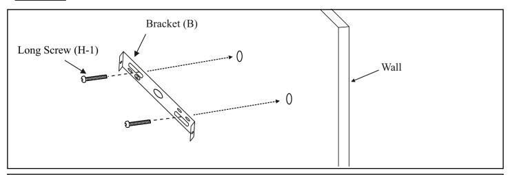
Align holes of Bracket (B) with the Wall Plug (H-3) and secure with Long Screws (H-1) using a Screwdriver (T-1; not included). Fully tighten, but DO NOT OVERTIGTHEN.
