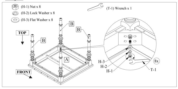
Place Tabletop (A) upside down onto a padded, non-marring surface. Align Legs (B) at each corner of Tabletop (A) making sure the hanger bolts install through the holes as shown. Secure each Leg (B) using Nut (H-1), Lock Washer (H-2), Flat Washer (H-3), stacking the hardware in the order shown. Fully tighten all Nuts (H-1) using the provided Wrench (T-1). DO NOT OVERTIGHTEN.
