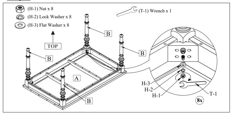
Place Tabletop (A) upside down onto a padded, non-marring surface. Align Legs (B) at each corner of the Tabletop(A) making sure the hanger bolts install through the holes as shown. Secure each Leg (B) using Nut (H-1), Lock Washer (H-2), Flat Washer (H-3), stacking the hardware in the order shown. Fully tighten all Nuts (H-1) using the provided Wrench (T-1). DO NOT OVERTIGHTEN.
