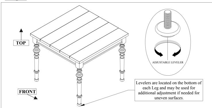
Using a second person to assist you, turn the assembled unit upright. Assembly is now complete and the product is ready for use. Adjustable levelers are located on the bottom of each leg and may be adjusted by turning outwards, counter-clockwise to help account for uneven surfaces.
