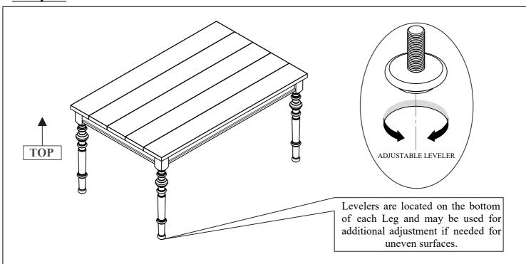
Using a second person to assist you, turn the assembled unit upright. Assembly is now complete and the product is ready for use. Adjustable levelers are located on the bottom of each leg and may be adjusted by turning outwards, counter-clockwise to help account for uneven surfaces.
