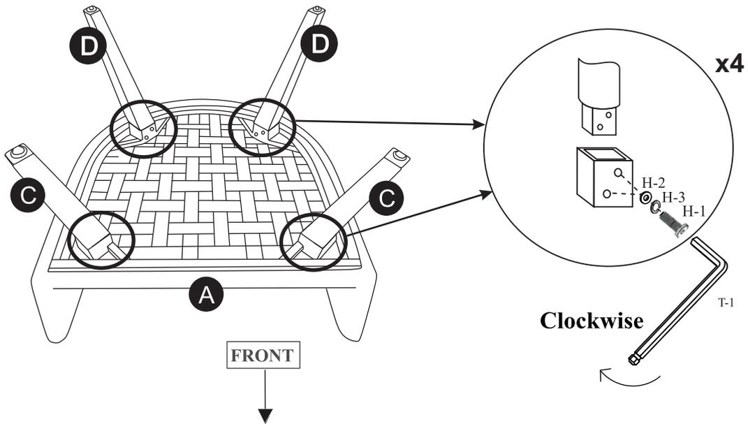
Place Seat (A) upside down onto a padded, non-marring surface. Position the Legs (C/D) in the correct locations based on the labels on the Legs (C/D) and Seat (A). Align all mounting holes. Secure Legs (C/D) to Seat (A) with Allen Bolts (H-1), Flat Washers (H-2) and Spring Washers (H-3) using provided Allen Key (T-1), stacking the hardware in the order as shown. Engage all Allen Bolts (H-1) first then fully tighten. Do not over tighten.
