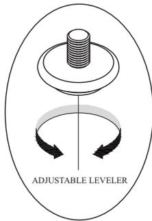
Levelers are located on the bottom of each leg and may be used for additional adjustment if needed for uneven surfaces.
