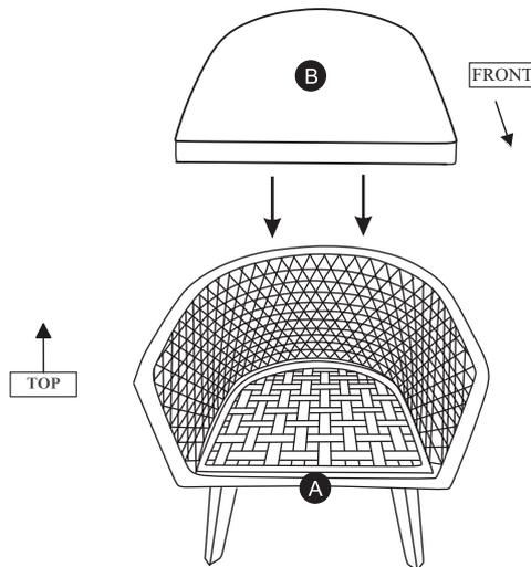
Carefully place assembly upright. Ensure it rests evenly on all four Legs (C/D). Ensuring it is oriented correctly, place the Cushion (B) onto the seat.
