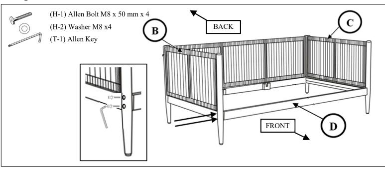
Position the Front Rail (D) to the front of the assembly. Ensure the cleats on the Front Rail (D) face toward those on the previously assembled Back Rail (E). Repeat the same process as step 1 to attach the Front Rail (D) to the Right/Left Panels (B/C).
