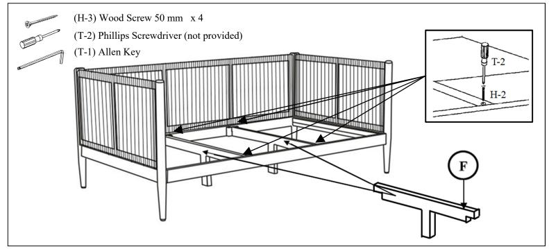
Position each of the two Middle Rails (F) by inserting the ends into the cleats located on the Front/Back Rails (D/E). Secure by engaging four Wood Screws (H-3) into each end and tighten using a Phillips Screwdriver (T-2; not included). Fully tighten ALL hardware from Steps 1-4 at this time using the provided Allen Key (T-1) and a Phillips Screwdriver (T-2; not included). DO NOT OVERTIGHTEN.
