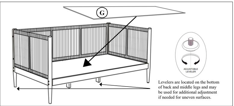
With the help of a second person, gently place the Mattress Panel (G) onto the assembly as shown. Carefully lift and move to your desired location.
