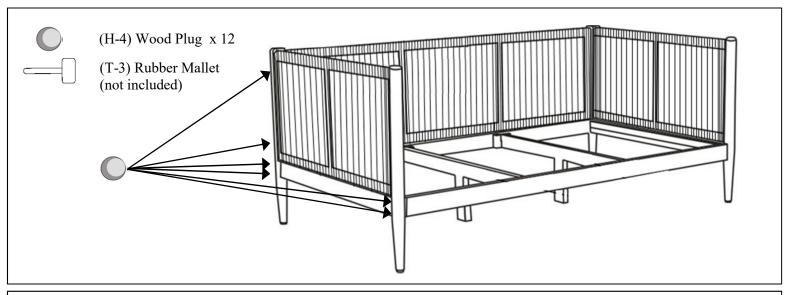
Insert the twelve Wood Plugs (H-4) into each hardware hole. Gently tap the Wood Plugs (H-4) with a Rubber Mallet (T-3; not provided) until they are securely fastened. DO NOT USE A METAL HAMMER WITHOUT PROTECTION, SUCH AS PACKAGING MATERIAL, BETWEEN THE HAMMER AND THE PLUG. It is highly recommended to use a Rubber Mallet.
