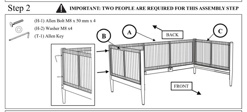
Very carefully, position the Back Panel (A) to the back of the assembly as shown. Ensure it is oriented correctly. Secure by engaging four Allen Bolts (H-1) and Washers (H-2) through each Side Panel (B/C). Tighten about 90% using the provided Allen Key (T-1). The assembly should be sturdy enough to now stand on its own, but do not bump or move the components to avoid breakage.
