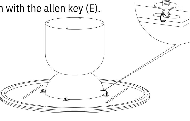
STEP-3 Adjust leveling feet to prevent tipping.
